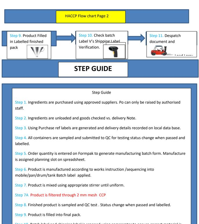
Step 10. Batch label and shipping label is scanned using comparator to ensure correct material is present vs. order requirement.
